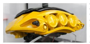
a cast aluminum caliper used on road cars. Topology optimization is a software tool that allows Brembo engineers to simulate the stiffness of a component and identifying the excess material. The result of this software, used for some time in the design of racing braking systems made from billet aluminum, is a new geometry that optimizes performance, stiffness and weight of the caliper."
